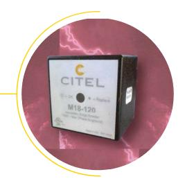
Citel's M40/M18 compact, low profile surge protectors are designed to protect local distribution panels, OEM control panels, PLC's, and SCADA systems against transient surge events. These devices are installed parallel to the AC network and provide robust surge handling capability. The M40 is available for all three phase applications and is rated at 40kA (8/20µs) transient amps per phase. The M18 is a single phase device with a transient amp rating of 36kA (8/20µs).
