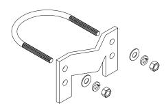
1) Remove hardware from U-bolt and remove U-bolt from bracket.
